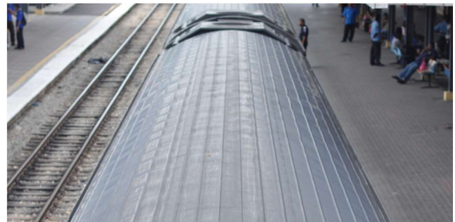
Figure 2. Longitudinal grooves on train roof (from [13]).
